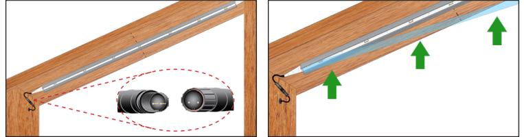
**Figure K. (LEFT)** Connect each set of flexible LED light strip to the jumper previously installed in each post.
