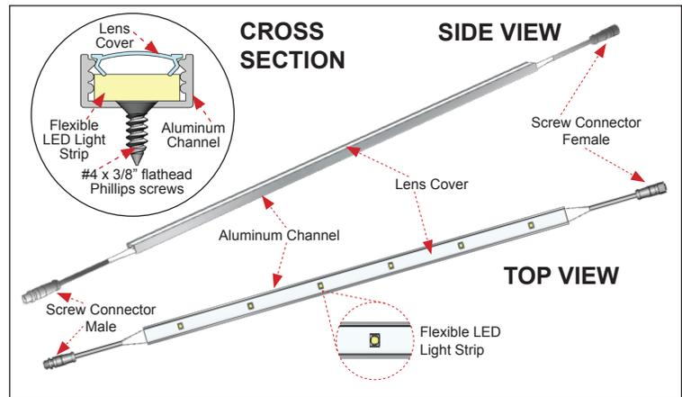
Figure A. Micro Star LED light bar.
