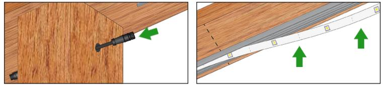
**Figure I. (LEFT)** Install the jumper (S0825-JMPR-SC) through each post.
